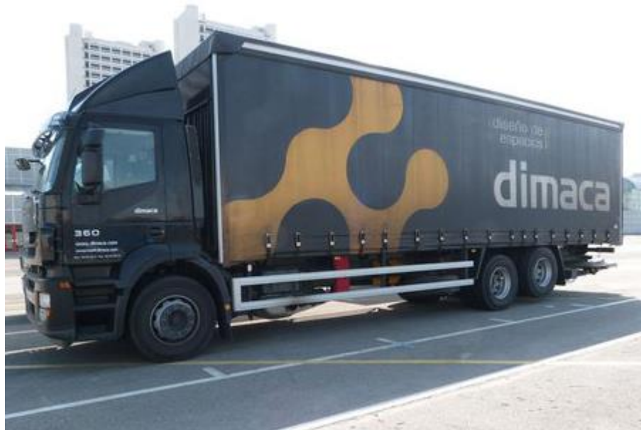
European Heavy Truck Equipped with a Side Guard (Image courtesy of Lloyd Alter )
