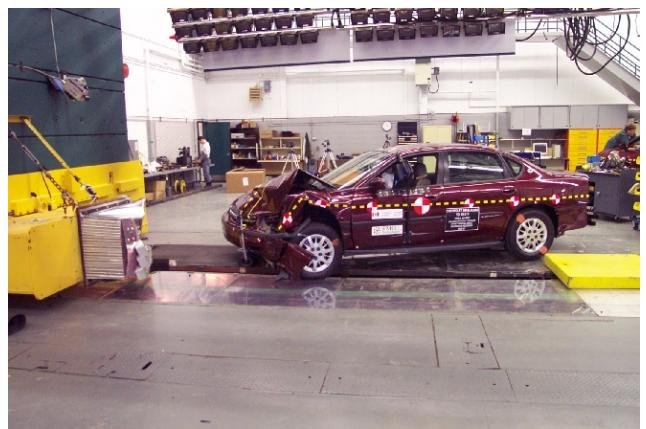
**Figure 2. Offset Deformable Barrier Crash Test**
