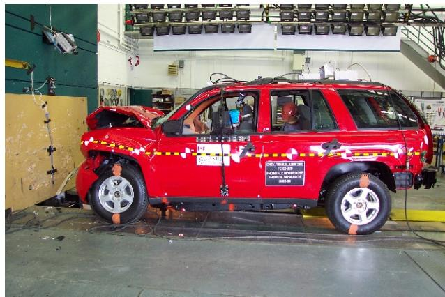
**Figure 1. Frontal Rigid Barrier Crash Test**
