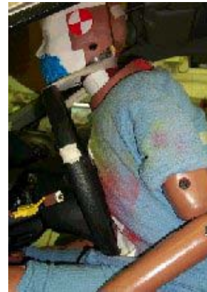
Figure 11. Chest-on-module out of position test
