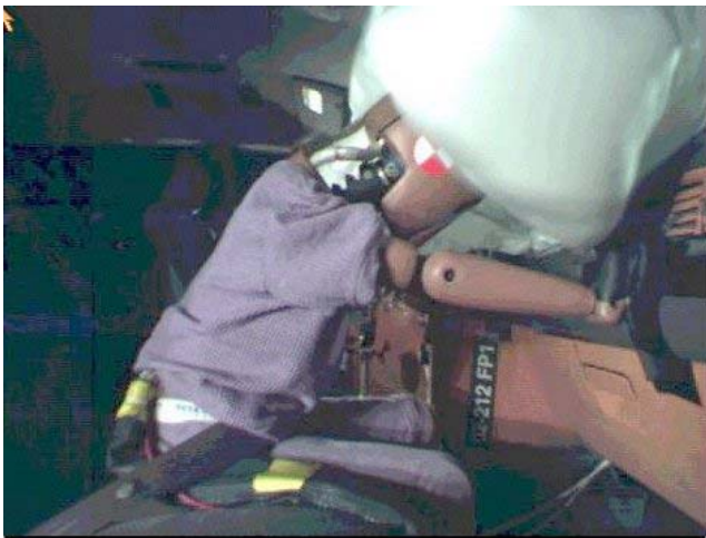
Figure 12. Air bag interaction with head of child dummy
