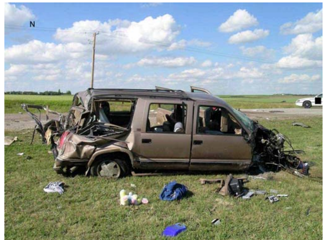
Figure 2: Damage to the D-Pillar Area of the 1995 GMC Suburban
