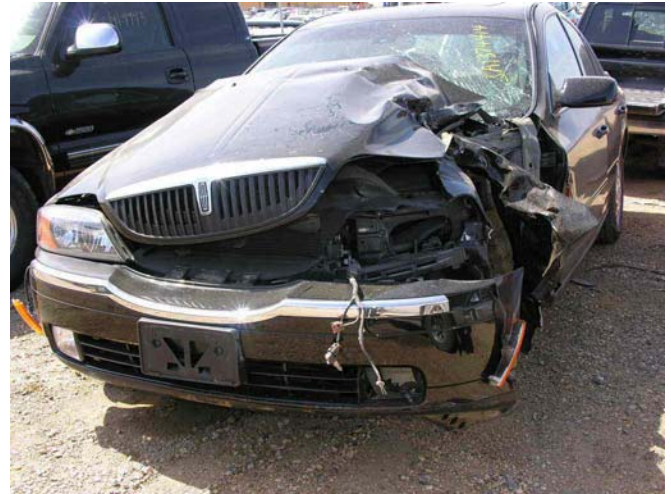
Figure 1: Damage to the Lincoln from the Honda Motorcycle
