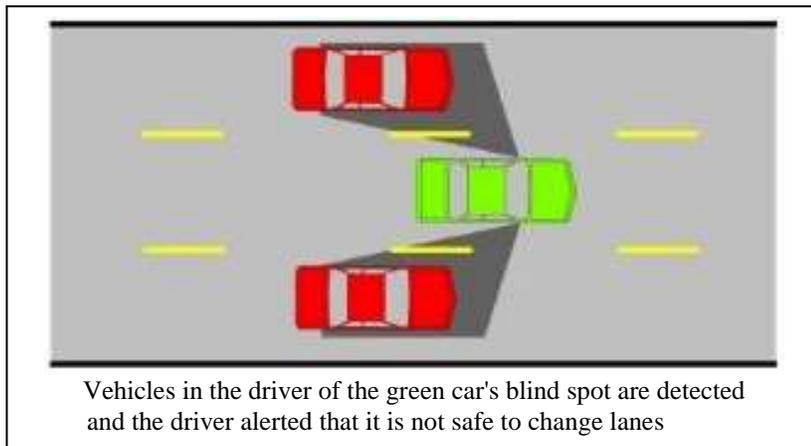
Generally, the system will illuminate a warning light, often located on the appropriate side mirror, to advise the driver of the presence of the adjacent vehicle. Other systems vibrate the steering wheel or seat if the driver attempts to initiate an unsafe passing manoeuvre.
